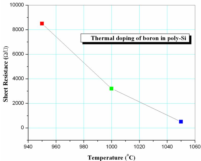
Fig 5: Measured Sheet Resistance for Different Doping Temperatures
