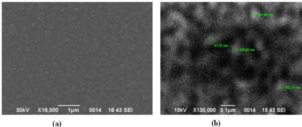
Figure 3: SEM image of polysilicon film.
